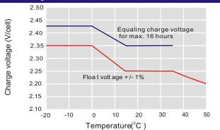
For continuous charging we recommend a voltage of 2.25 V. The charging voltage must be compensated to the curve for acontinuously different battery ambient temperature.
